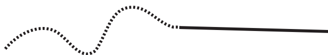
Figure 1. Schematic illustration of a rod-coil copolymer chain. The full (broken) line indicates the rod (coil) block.
